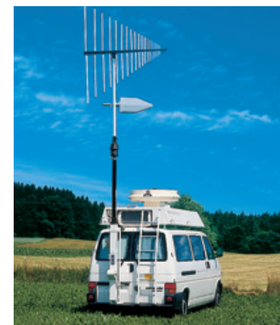
You can also locate interferers by using mobile units, for example when operating in the bands of mobile radio networks or other radio services.
