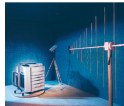
Large units such as photocopiers also have to undergo EMC testing in anechoic chambers.
